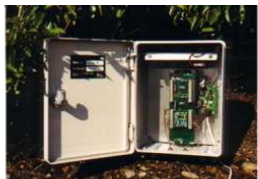
The new DataTrek logger, complete with modem extension board
